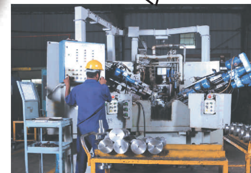
Oil Hole Drilling
