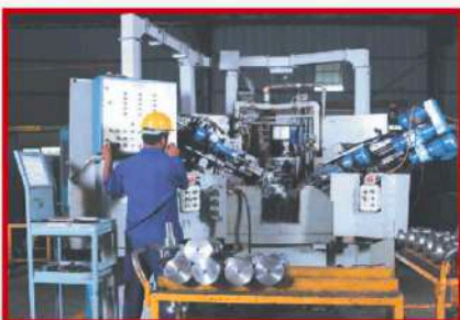
OIL HOLE DRILLING
